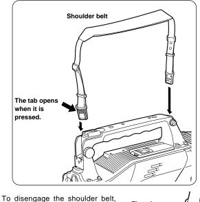
To disengage the shoulder belt, open the tabs of the attachment parts, and disengage. The tab opens when it is pressed.
