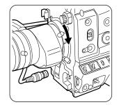
**4** Push the cable into the cable clamp, and connect it to the LENS jack.
