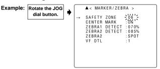
4 Rotate the JOG dial button to change the setting, and press the JOG dial button at the desired setting. The setting is now entered.
