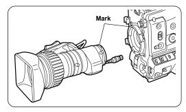
${f 3}$  Pull down the lens lever to secure the lens.
