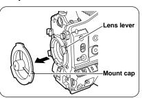
2 Fit the center mark on the lens into the center cutout on the top of the lens mount, and attach the lens.
