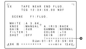
Status displays on the viewfinder screen when the MODE CHECK switch is ON (FULL AUTO)
