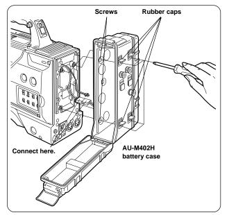
**3** Connect the plug of the battery pack to the connector inside the battery case, and insert the battery pack into the case.
