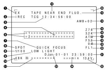
Status displays on the viewfinder screen when the MODE CHECK switch is ON (normal)
